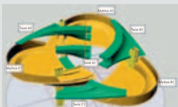
Schematic 3D presentation of the Mythos segment (yellow), Twist (green) and satellite cores (light green).
