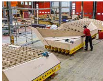
PERI provides customised 3D boxed elements for the construction of complex, multi-curved reinforced concrete components.
