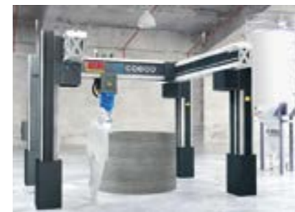
Configuration example with one X-axis module, two Y-axis modules and one Z-axis module respectively (consisting of four Z-axes).
