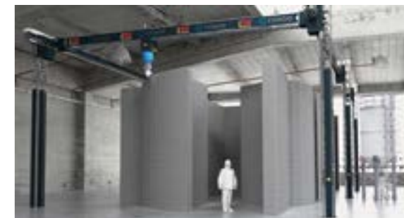
Configuration example with four X-axis modules, eight Y-axis modules and three Z-axis modules respectively per Z-axis.
