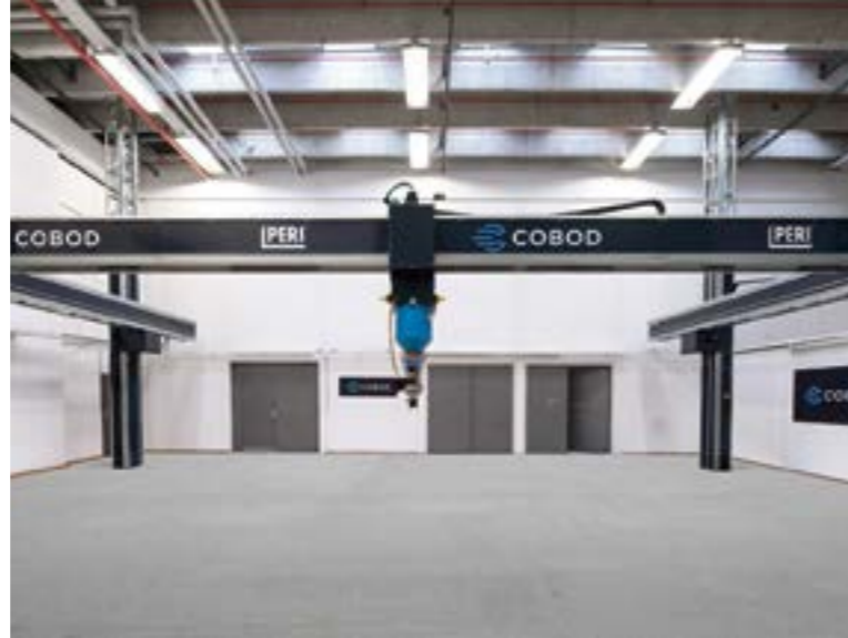
The BOD2 is a modular printing system. Thanks to the 2.50 m long modules, it can be flexibly mounted in any direction.
