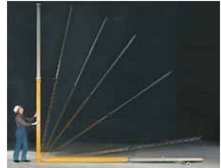
In drop tests on a transversely positioned steel tube, an extended MULTIPROP Prop remains completely undamaged – in contrast to, e.g. tubular steel props.
