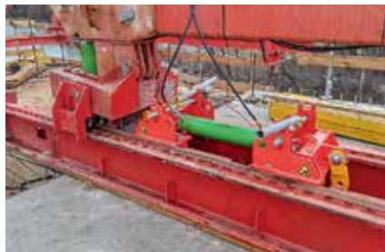
No unintentional movement The equipment is always mechanically secured when being moved forward to the next cycle.
