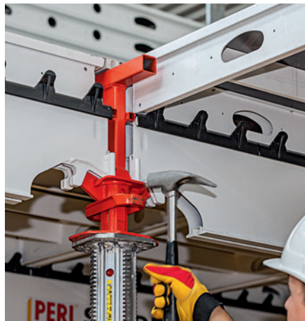
Easy and simple early striking: the formwork is lowered by 6 cm with just one blow of the hammer.
