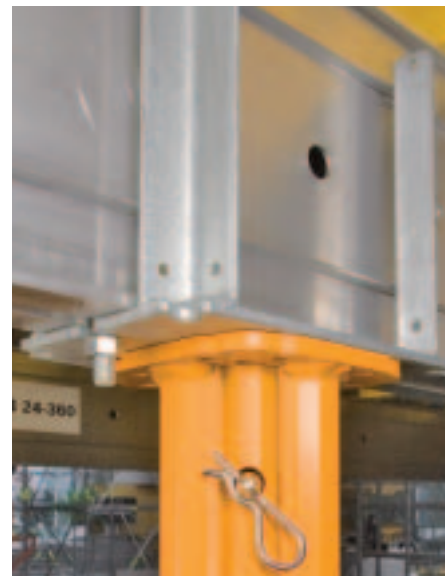
For use as tables, the MBP 24 beam is secured to the crosshead by means of the MP Bolt with Nut (Item no. 111142). The crosshead is mounted to the MULTIPROP using Pins \varnothing 14 x 107, galv. (Item no. 027990) and Cotter Pins 4/1 (Item no. 018060).
